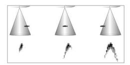
Transducer Cone and Fish Arches
